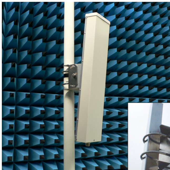
stainless steel rear bracket with downtilt
