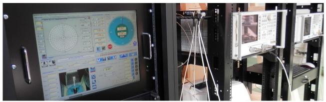
After the prototypes have been made, the delicate antenna characterisation phase begins. These measurements define the behaviour of the antenna, and it is clear that it is indispensable to perform them correctly.
