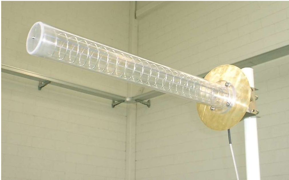
Figure 4.1 Axial mode helical antenna for the 1400÷1650 MHz band.
